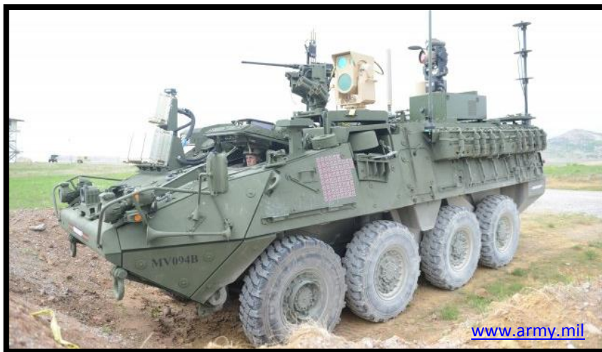
This Mobile High-Energy Laser-equipped Stryker was evaluated, April 12, during the 2017 Maneuver Fires Integrated Experiment at Fort Sill, Oklahoma. The MEHEL can shoot a drone out of the sky using a 5kW laser. (Photo Credit: C. Todd Lopez)
